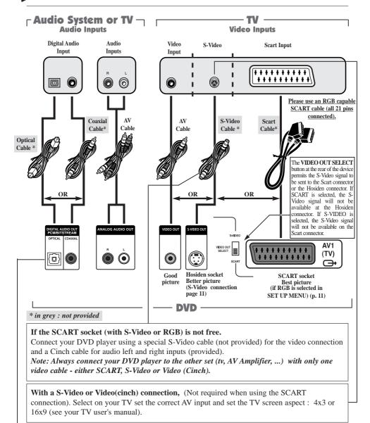
Remove the protection cap from the DVD socket and connect the optical audio digital cable firmly as shown.
